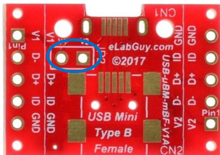
Figure 5: PCB front with open circuit on VCC pin in series
